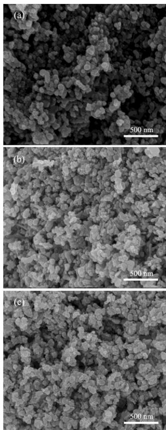
**Figure 2.** SEM images (a)ZnO; (b)ZnO-Ga-49:1 (c) ZnO-Ga-27:1
