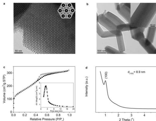
**Figure 1.** (a,b) Typical HRTEM images of ordered mesoporous  $g\text{-C}_3\text{N}_4$ @CMK-3 nanorods. Inset in panel a represents a schematic illustration (yellow:  $g\text{-C}_3\text{N}_4$ , black: carbon); inset in panel b reveals the ordered mesoporous channels. (c) Nitrogen sorption isotherm at 77 K with the corresponding pore size distribution (inset) and (d) low-angle XRD pattern of  $g\text{-C}_3\text{N}_4$ @CMK-3.
