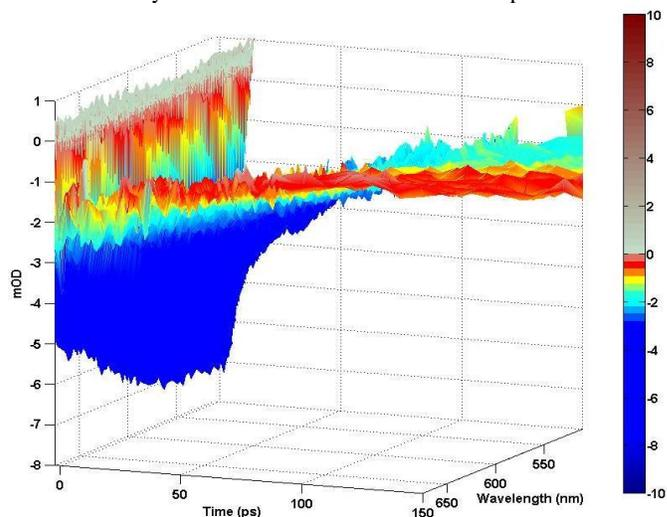
**Figure 1.** Transient absorption decay profile of H<sub>2</sub>-treated TiO<sub>2</sub> nanowires following a 470 nm pump excitation with a white-light continuum monitoring probe. Following the initial 180 fs excitation pulse, electron-hole recombination as well as electron trapping into trap states occur quickly (~5 ps), which is followed by slower trapping/recombination events persisting to tens of picoseconds.
