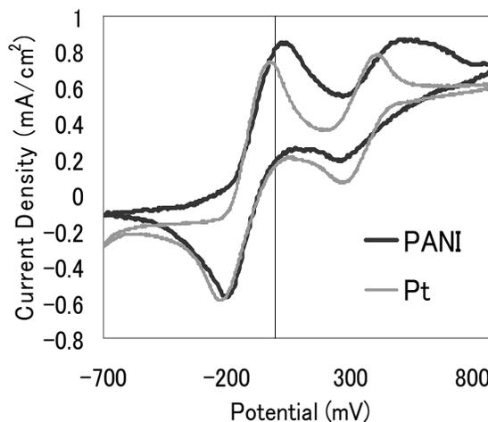
Figure 1. Cyclic voltammogram for Pt and PANI electrode
