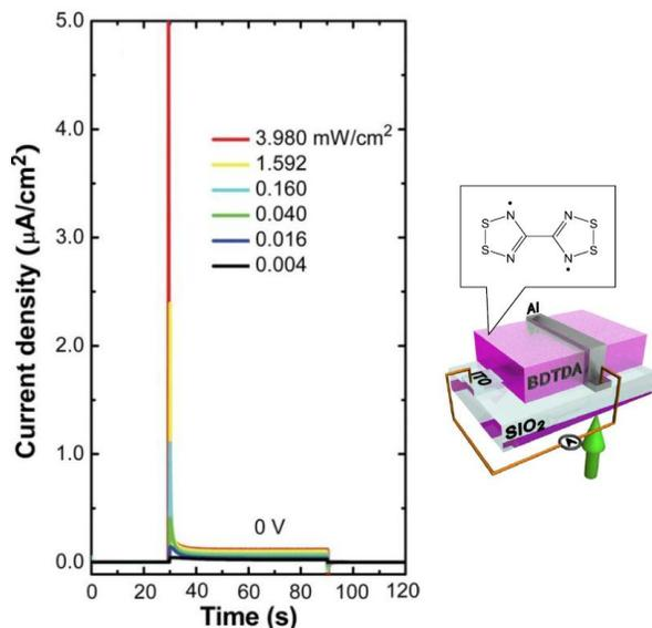
**Figure 1.** Photoresponse of an ITO/BDTDA (300 nm)/Al photocell (inset) under an illumination of a green laser (532 nm) under vacuum with a bias voltage of 0 V.
