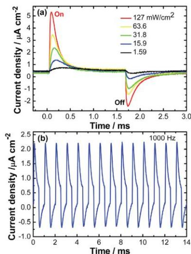
**Figure 2.** The photoresponse of an ITO/PVDF/ZnPc:C<sub>60</sub>/Al photocell under illumination from a modulated 532-nm laser (300 Hz) with different intensities. The sample was illuminated from the ITO side. (b) Photoresponses with a light modulation of 1 kHz.
