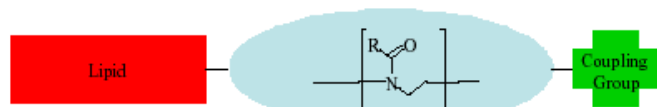
Figure 1. Cartoon of the 2-alkyl-2-oxazoline lipopolymer with a lipid head group, a hydrophilic polymer spacer and a silane coupling end function.
