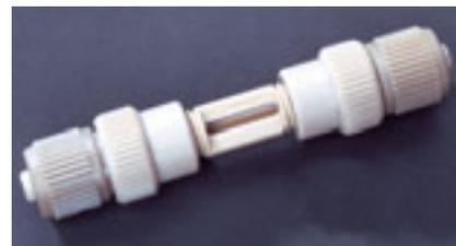
**Column.** This capillary sample trap column is ideal for preconcentrating low-level samples or removing impurities from low-concentration samples before injection. It features a fused-silica capillary column and incorporates a 1-µm filter with only 10 nL of swept volume.
