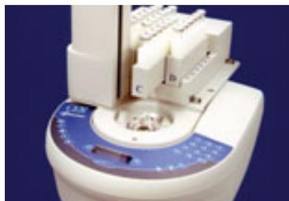
**Workstation.** This fully automated synthesis system features parallel throughput with sequential reaction control. The workstation is small enough to fit in a fume hood, and its 24-sample deck has interchangeable racks for unlimited capacity.
