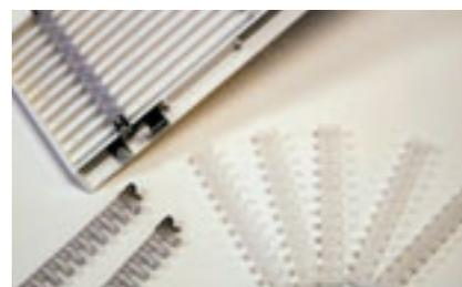
**Sample loading.** This cup-loading option enables easy loading into rehydrated IPG strips on an isoelectric focusing system. It is ideal for the separation of proteins at extreme pH ranges and has better resolution during first-dimension isoelectric focusing. The convenient, disposable cups are available in strips of 12 in 100- or 150-µL volumes.
