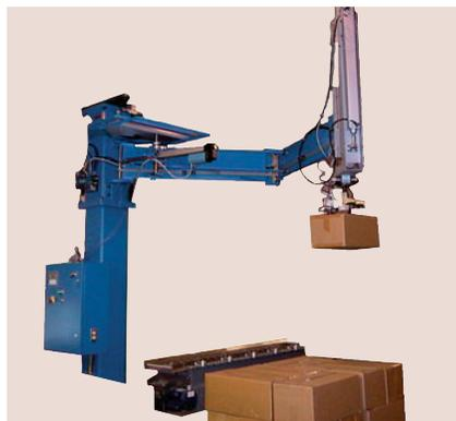
**Robotic arm.** The Stackbot is controlled by a track plate rather than a personal computer, ensuring that a programmer or a skilled technician is not needed for new pallet patterns. A 2-min swap of a track plate creates the new pattern, and the robot can load or unload two different pallet patterns simultaneously in an area smaller than that required for current manual loading. It palletizes or depalletizes up to 10 cases (pails, bags, bales, or trays) per minute.
