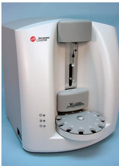
**Cell viability analyzer.** The Vi-CELL automates the widely accepted trypan blue tissue culture protocol. Compared with manual techniques, the number of cells that the analyzer counts is significantly greater, and results are obtained in minutes.
