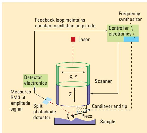
**Figure 1. Atomic force microscopy.** The schematic shows the feedback loop for tapping-mode operation.
