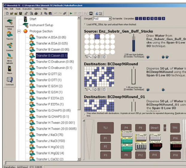
**Figure 1. Example of a liquid-handling method and deck layout from AAO on a Biomek FX. Each highlighted source has its associated destination plate map displayed for verification while the liquid handler is active.**
