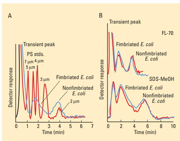
**Figure 2. Bacterial separation.** (A) Using asymmetric flow FFF, fimbriated and nonfimbriated *E. coli* are separated, and their sizes are compared with internal (PS) standards. (B) The retention profiles of the bacteria change when two different carrier solutions are used: FL-70 and SDS-methanol (MeOH). (Adapted with permission from Reschiglian, P.; et al. *Anal. Chem.* **2002**, *74*, 4895–4904.)
