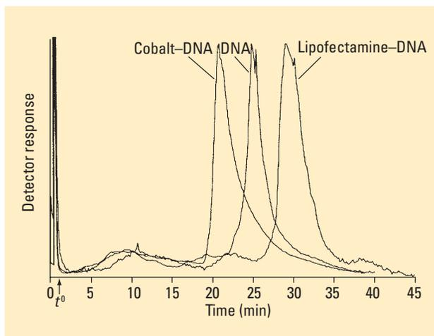
**Figure 3. Macromolecule fractionation.** Researchers used flow FFF to characterize plasmid DNA and DNA complexes. (Adapted with permission from Lee, H.; et al. *Anal. Chem.* **2001**, *73*, 837–843.)
