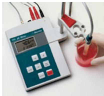
**pH Meter.** This instrument has a large LCD display and step-by-step procedure icons. The measuring ranges are  $-0.00$  to  $14.0$  pH,  $-2000$  to  $2000$  mV, and  $-170.0$  to  $199.90$   $^{\circ}\text{C}$ . Temperature, drift, and direction are visible during measurement, and up to nine pairs of pH or mV-temperature valves can be stored on demand, at selected time intervals, or when the reading is stable.
