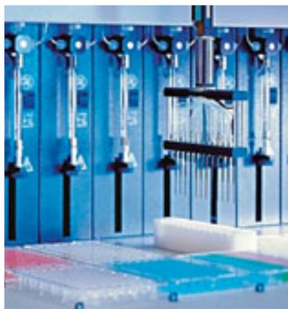
**Workstations.** The 4000 MPH series of instruments and the Microlab Star can perform sample normalization with Vector control software. Vector software accepts data from various plate reader manufacturers, calculates volumes, and creates appropriate pipetting sequences during run time. One
