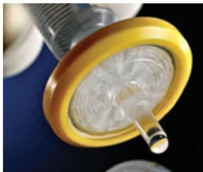
**Syringe filter.** The Millex 33-mm syringe filter with Durapore PVDF Membrane is used for the sterile filtration of antibiotics, media preservatives, and protein-containing solutions. It offers nearly 20% more surface area than traditional 25-mm syringe filters, increasing flow rate and throughput and accelerating filtration. The filter has a maximum housing pressure of 150 psig (10 bar) and is available in 50 and 250 packs with pore sizes of 0.1, 0.22, and 0.45  $\mu\text{m}$ .
