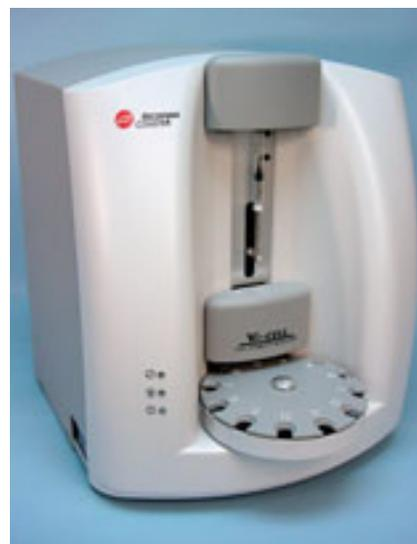
**Cell viability analyzer.** The Vi-CELL automates the widely accepted trypan blue tissue culture protocol. Compared with manual techniques, the number of cells that the analyzer counts is significantly greater, and results are obtained in minutes.
