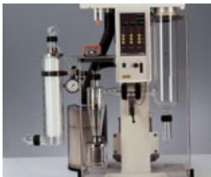
**Spray dryer.** The Büchi spray dryer B-191 produces dry, uniform powders from 50 to 100 mL of solution in 10 min. The microprocessor-controlled heating system ensures that the desired inlet remains constant even when the drying air flow rate changes. Applications include spray drying, micronization, microencapsulation, and recovery of synthetic and extracted products.
