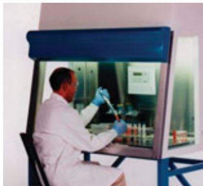
**Cabinets.** The class II Heraeus HERASafe KS safety cabinets provide product and personnel protection through their ergonomic design. They feature a slanted front window, rear cabinet wall, digital eye-level display, and remote control. The information displayed includes downflow rate, total operating hours, time of day, and optional UV-C irradiators' operating time. The display also has a stopwatch function. The work aperture has a height of 10 in.
