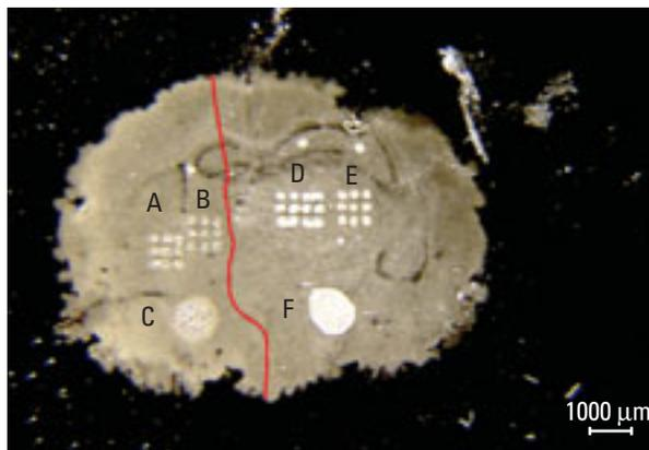
**Figure 2. Mass appeal.** A cross section of a juvenile mouse brain whose left side was seeded with matrix crystals and then spotted with MALDI matrix by acoustics (A, B, D, E) and pipette (C, F). The acoustic transfers involved 15 (B, E) and 30 (A, D) 120-pL droplets, forming spots ~170  $\mu$ m in diameter. The pipette transfers were 100-nL formatting spots ~1000  $\mu$ m in diameter. (Adapted with permission from Ref. 6.)
