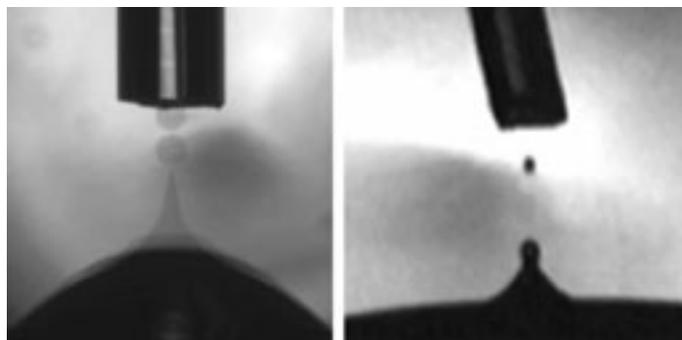
**Figure 1. The sound and the flurry.** Researchers at Labcyte Inc. have developed a liquid-handling method that harnesses sound energy to project sample droplets at small capillaries. (Adapted with permission from Ref. 6.)
