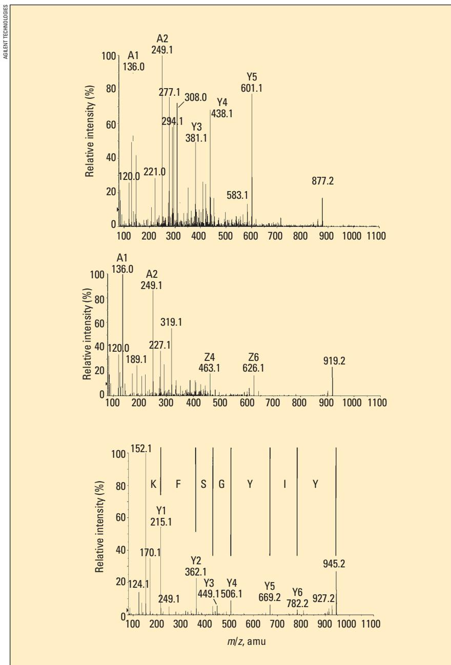
**Figure 3. MALDI MS/MS of a standard peptide with the sequence YYIGSFK.** Spectrum of the standard peptide (top), the peptide derivatized with *O*-methylisourea (middle), and the peptide derivatized with 2-methoxy-4,5-dihydro-1*H*-imidazole (bottom). The latter derivative yields an uncomplicated series of  $\gamma$ -ions that facilitates identification of the peptide sequence.
