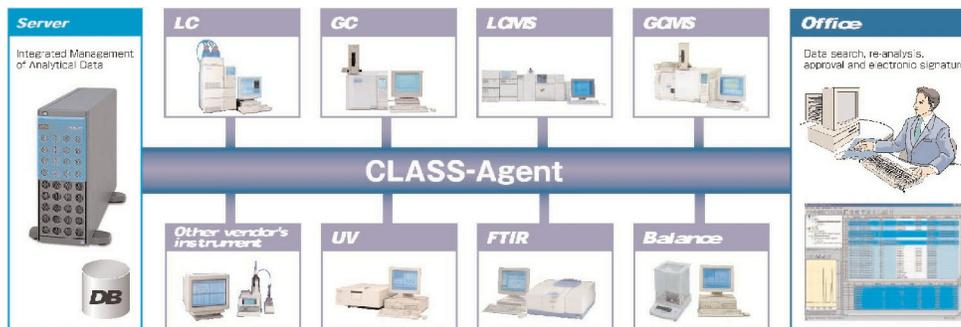
**FIGURE 1:** By interfacing analytical instruments with a central network, researchers can use the devices and analyze the data from any computer attached to the system. Also, data can be stored easily and efficiently on a central server, simplifying regulatory compliance. (Image courtesy of Shimadzu Scientific Instruments.)
