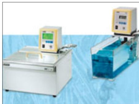
**A Lauda Ecoline stainless steel heating bath/circulator (left) and immersion circulator (right).**
