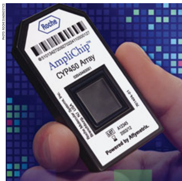
Clinical array? Roche's AmpliChip CYP450 may soon be the first DNA microarray approved as an in vitro diagnostic device.
