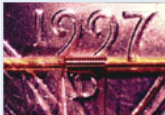
Small change. Microcoil NMR probe and a penny. (Adapted with permission from Peti, W.; et al. J. Am. Chem. Soc. 2004, 126, 5873–5878.)
