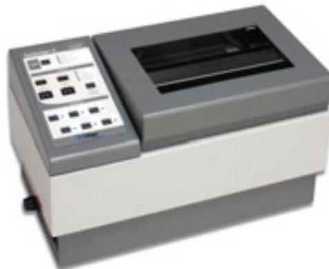
Nitrogen blowdown evaporator. (Photo: Caliper.)
