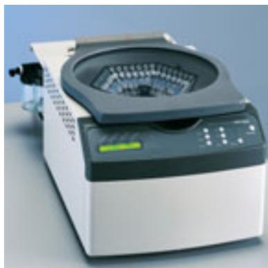
A centrifuge evaporator. (Photo: Labconco.)
