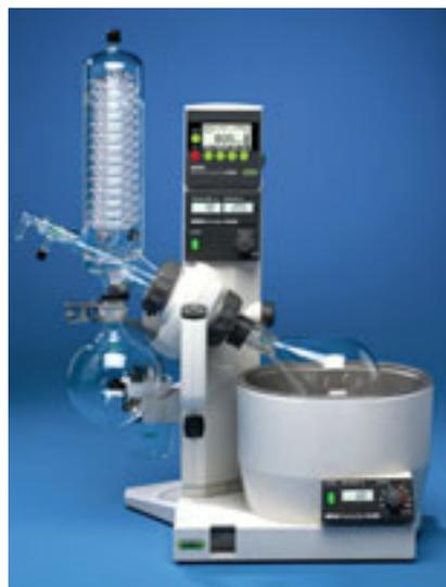
A rotary evaporator. (Photo: Brinkmann Instruments.)
