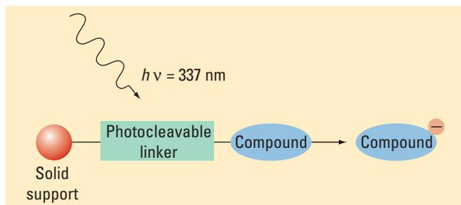
**Broken link.** Photocleavable linkers can be used for direct MS monitoring of solid-phase organic synthesis (Adapted with permission from Gerdes, J. M.; Waldmann, H. *J. Comb. Chem.* **2003**, *5*, 814–820.)
